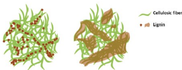
615 616 Fig. 8 Proposed model to describe the location of the lignin within LCNF suspension after filtering 617 (left) and LCNF nanopaper after pressing (right) Reprinted and adapted from Rojo et al. (2015) 618 with permission of Royal Society of Chemistry.
