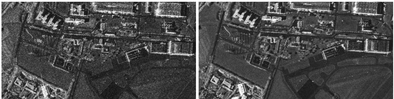
Fig. 14. Geocoded zoom of the scene shown in Fig. 13 for the (left) operational HS mode and the (right) ST mode. The resolution of the multilooked images in both cases is approximately 1 m. Zoom size: 1000 m × 500 m.
