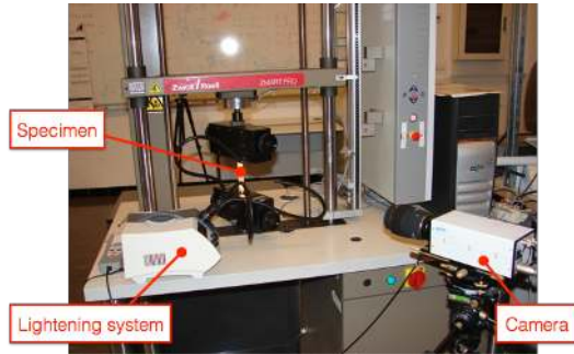
(a) Illustration of the set-up with its instrumentation (camera and lighting system)
