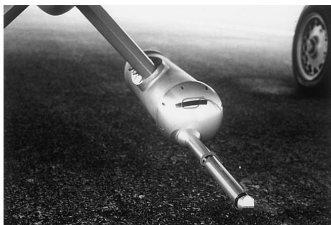
Fig. 1. Ice replicator mounted on the DLR research aircraft 'Falcon'
