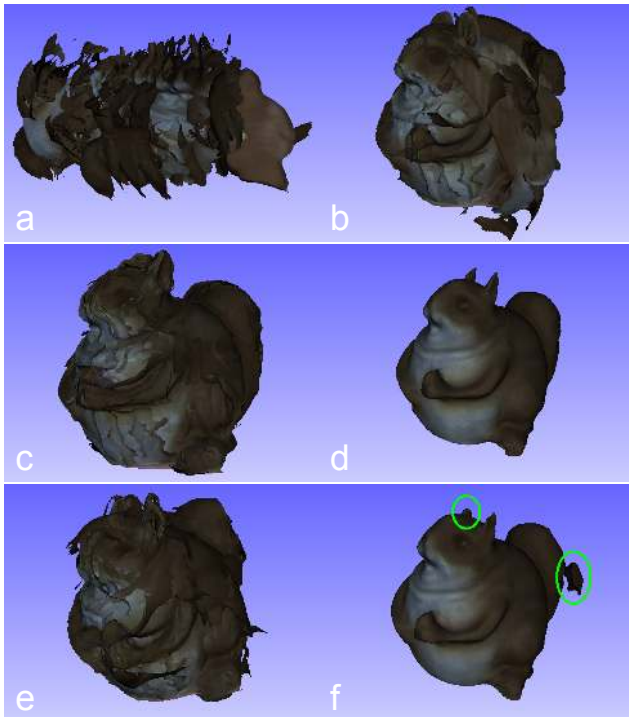
Figure 8. 3D reconstruction based on the SHOT descriptor: (a) initial views. (b) coarse registration with SHOT LRF (c) coarse registration and (d) reconstruction with the proposed LRF (e) coarse registration and (f) reconstruction with PS LRF. A 3D visualization of the results is provided in the supplementary material.
