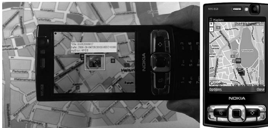
Figure 2. (Left) MapLens in use with a paper map, overlaying digital information on screen. With the red square (center) user locates and selects markers—as one user states—“catches them.” (Right) DigiMap version, Google map with markers.
