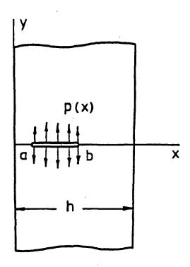
Fig. 1 A Crack in an Infinite Strip
