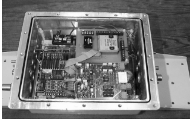
Figure 5.6: The Imagenex control box. This self contained module can be connected to a PC or the vehicle and allows the development of sonar processing algorithms independently of the submersible.
