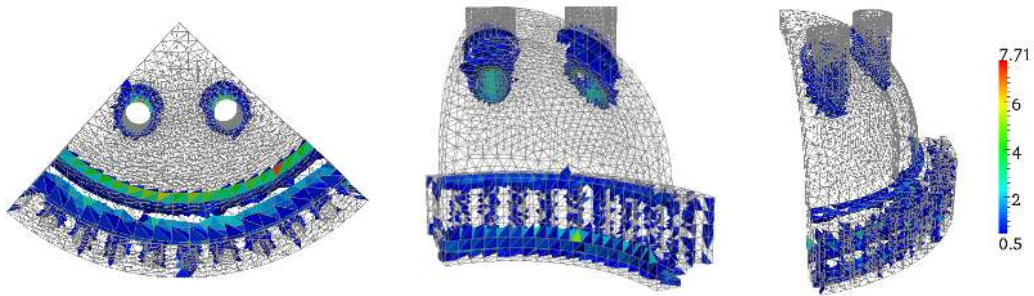
Figure 21. Spatial distribution of relevant local contributions to the density of the energy norm of the reference error.
