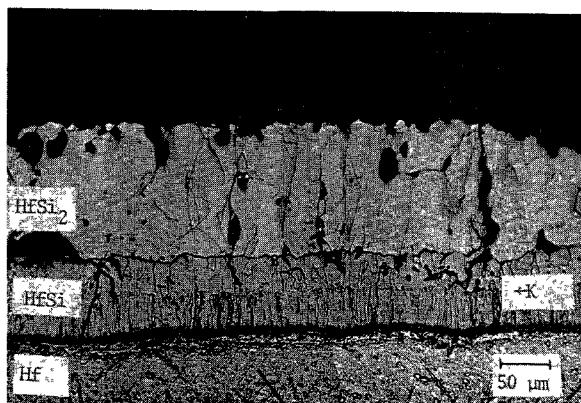
Fig. 5. Hf-HfSi<sub>2</sub> diffusion couple annealed for 24 h at 1523 K; K denotes the position of the Kirkendall interface.
