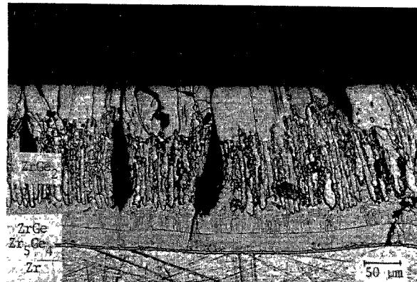
Fig. 7. Zr-ZrGe<sub>2</sub> diffusion couple annealed for 23 h at 1493 K.
