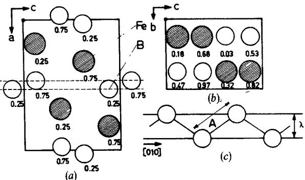
Fig. 1. FeB structure (Schubert, 1964), orthorhombic,  $D_{2h}^{16}$ ,  $Pnma$ .
