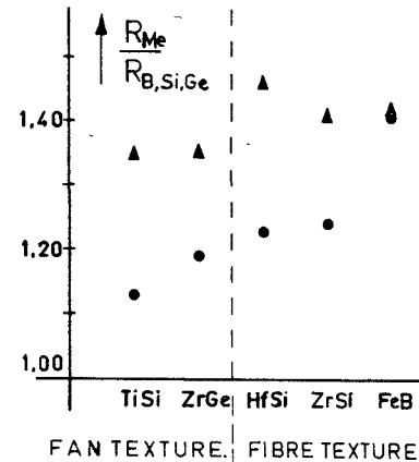
Fig. 8. Ratio of atomic radii in compounds with the FeB structure.
