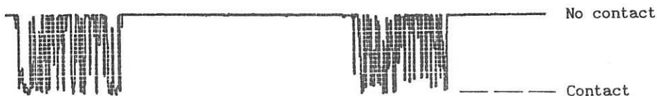
Fig. F2: Contact "resistance" measurement.
