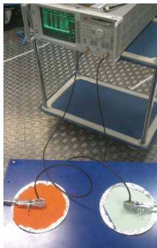
Figure 3. Two 10 cm monopole antennas with ground plane and an Agilent E8364BD network analyser for the measurement of the S_{21} parameter of the tank.
