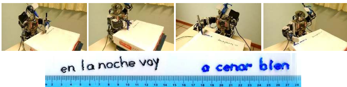
Figure 15. Transcription of a long sentence with the Bioloid's left and right arm and the kinematic models ( r = 0.3 cm)
