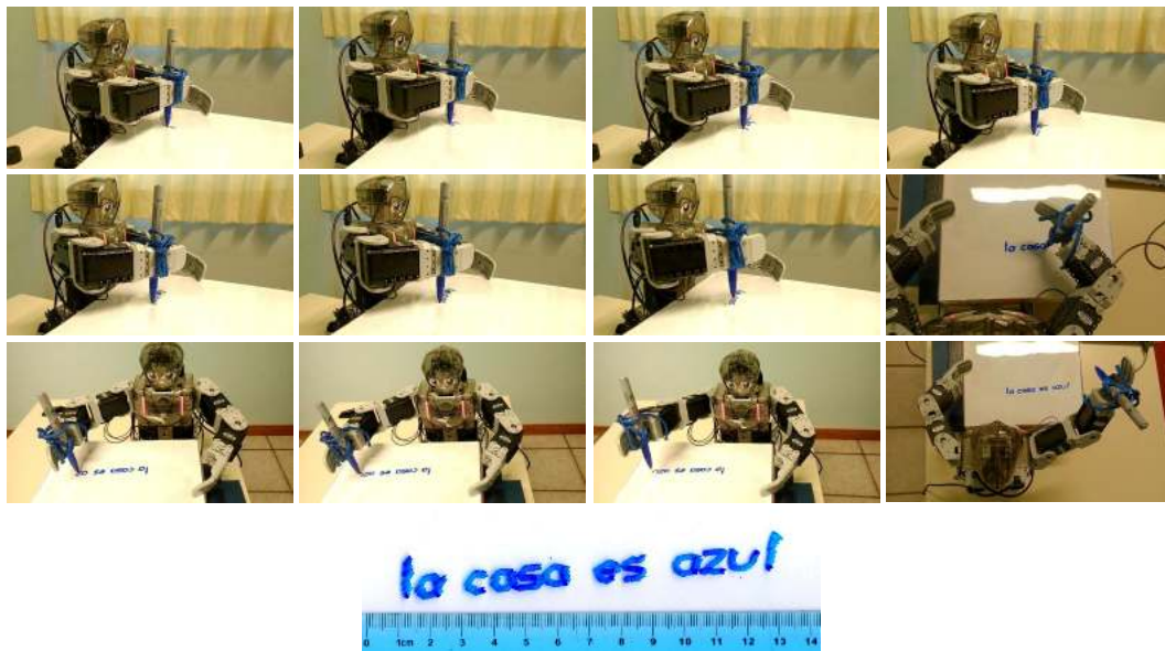
Figure 14. Transcription of a short sentence with the Bioloid's right arm and the kinematics models ( r = 0.3 cm).
