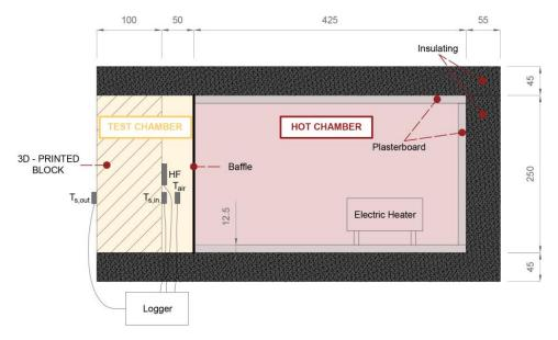
Figure 5. Configuration used for the HFM analyses.
