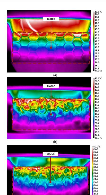
**Figure 10.** Thermal images—top view. (**a**) Block with wood sawdust. (**b**) Block with sheep's wool. (**c**) Block with hemp.
