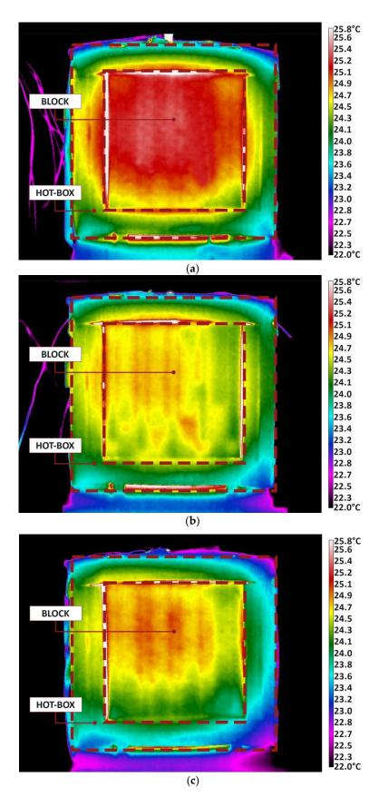
**Figure 9.** Thermal images—front view. (**a**) Block with wood sawdust. (**b**) Block with sheep's wool. (**c**) Block with hemp.
