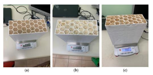
**Figure 4.** Weight of the three samples. (**a**) Block with wood sawdust. (**b**) Block with sheep's wool. (**c**) Block with hemp.
