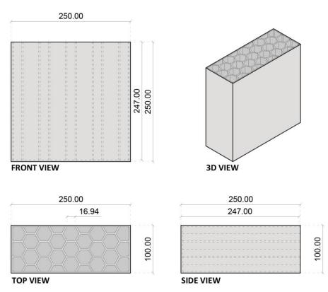
**Figure 2.** 2D and 3D block design (measurements in millimeters). Remark: PLA thickness is equal to 3 mm.
