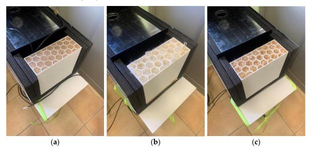
**Figure 7.** The three samples placed inside the Hot Box. (**a**) Block with wood sawdust. (**b**) Block with sheep's wool. (**c**) Block with hemp.
