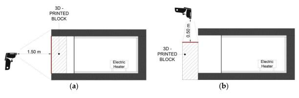
**Figure 6.** Configuration used for the IRT technique. (**a**) IRT technique in front of the block. (**b**) IRT technique from the top of the block.
