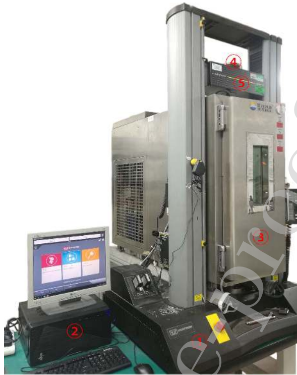
Figure 2: A complete thermo-viscoelastic testing system: (1) is the main framework of the Instron 5567, (2) is the control computer, (3) is the temperature chamber, (4) is the force transducer to monitor the applied force, and (5) is the crosshead of (1)
