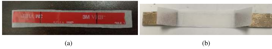
Figure 1: Specimen preparation. (a) Step 1: VHB tape with a required length is attached to a clean silicon paper, (b) Step 2: after removal of the red protective surface of VHB
