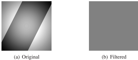
Fig. 2. Illustration of line zero moments as an edge annihilator. The piecewise polynomial image in (a) was filtered with a 2-D filter C(z_1, z_2) = (1 - z_1 z_2^2)^3 . The output image (b) pixels are approximately zero.
