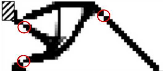
Figure 5. An optimal topology for a compliant gripper from F13 (Deepak et al., 2009).
