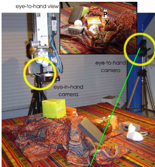
Fig. 6. Experimental setup: the scene is complex and the background is textured. The two camera locations are highlighted. Top right, the eye-To-Hand view is display with the clicked point {}^c p . The green line represents the line of view associated with {}^c p
