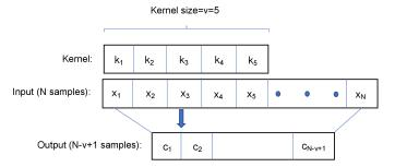
Fig. 4: Illustration of convolution operation at conv1D layer.
