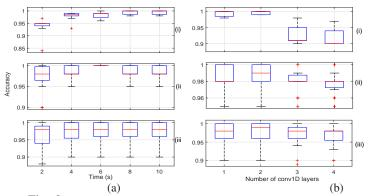
Fig. 8: Illustrates average classification accuracies for (a) varying lengths of input signal and (b) varying number of conv1D layers in: (i) database K, where the accuracies are shown with respect to pair-wise mental task classification, (ii) and (iii) databases E and R with respect to all the subjects respectively.
