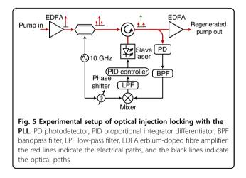
At the receiver, the pump was separated from the signal-idler path for regeneration purposes using a WDM coupler (at a 0.1-dB loss). For the recovery of the very weak pump, we applied an EDFA pre-amplified injection-locking (IL) scheme with an electrical PLL, as shown in Fig. 5, capable of recovering a stable pump at input powers as low as -72 dBm, which was 12 dB below the measured signal plus idler power<sup>15</sup>.
