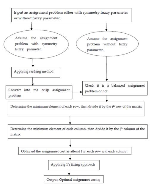
Figure 3. Architecture of the proposed algorithm.
