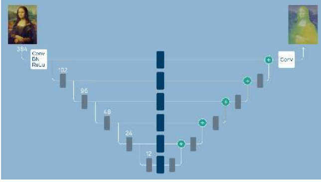
Fig. 2. Depth estimation network schematic. Gray TR blocks are used in down-/up-sampling passes and blue TR blocks are used to preserve spatial resolution. TR Blocks are defined in Fig. 3
