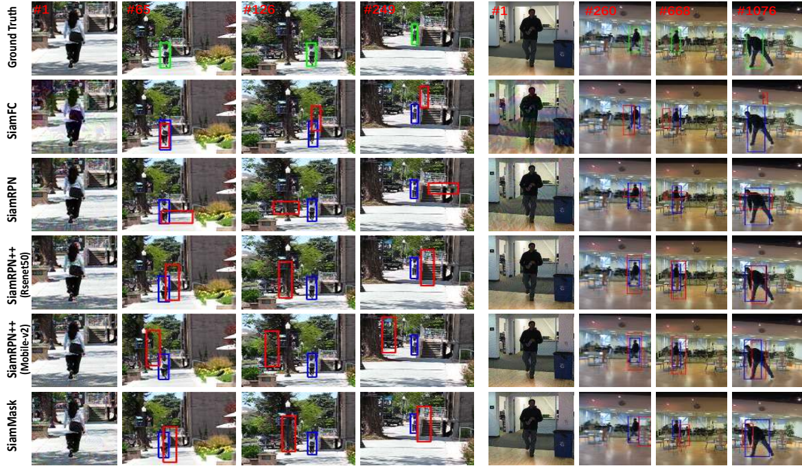
Figure 4. Qualitative evaluation of one-shot adversarial attack in various trackers on video examples Human7 and Human2 from the OTB100 dataset. For each of the two subfigures, the first column represents the adversarial examples generated in the initial frame, except the clean example in the first row. The green, blue, and red rectangles represent the bounding boxes of ground-truth, tracking results before and after being attacked.
