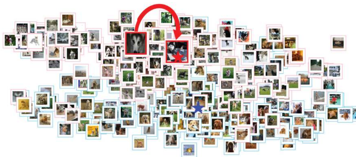
Figure 2: 2D visualization of image features for one-shot classification of two classes, namely Alaskan Malamute (framed in pink) and Golden Retriever (framed in blue). After restoration, the original prototype of Malamute (framed in red, left) is moved to the right, which is closer to the class center (marked by the red star). We visualize the shifted prototype (right) using its nearest real image. The figure is plotted by applying t-SNE of ResNet18 features of samples from miniImageNet . Best viewed in color.
