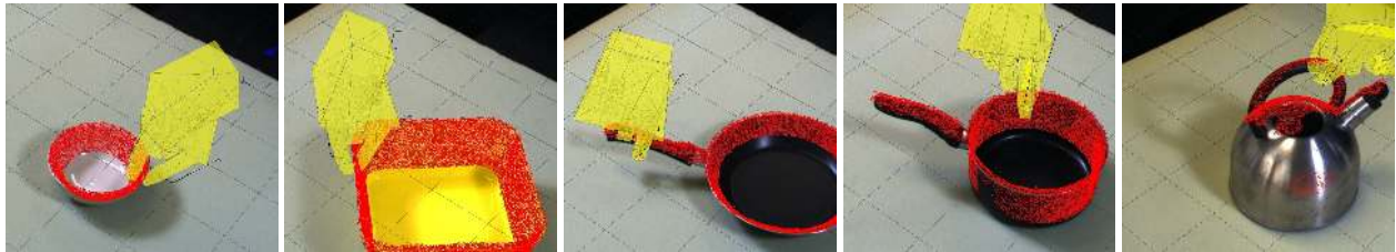
Fig. 10. The test objects with a visualisation of five of the failing grasps. The left four are from the 7 view condition and the kettle is from the 1 view condition.
