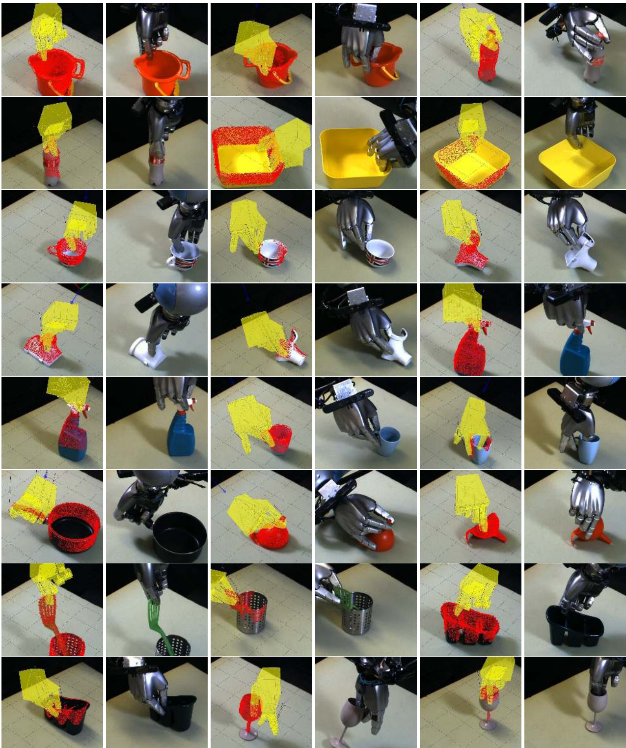
Fig. 9. The test objects with a visualisation of some of the successful grasps. Each grasp is shown by a pair of images, with the visualisation of the planned grasp and the obtained point cloud on the left, and the actual grasp execution on the right. Those from the 7 view and 1 view conditions can easily be distinguished by the proportion of the object covered by the recovered point cloud.
