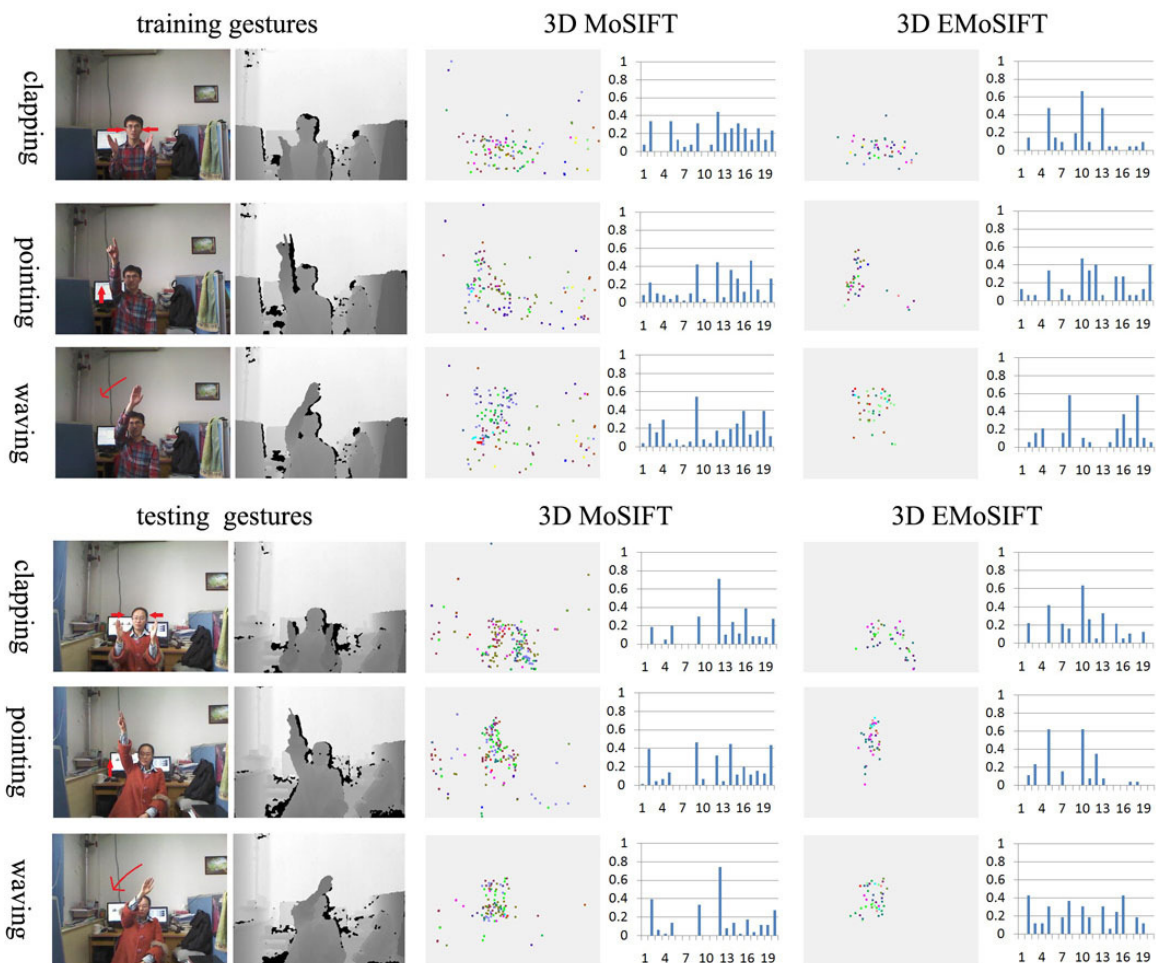
Figure 15: The first two columns are the samples used for training and testing. The third and fifth columns reveal the spatial distribution of the visual words for the samples, which show 3D EMoSIFT is more compact. We superimpose the interest points in all frames into one image. Different visual words are represented by different colors. The fourth and sixth columns are shown the histograms for each sample. The histogram vector is \ell_2 normalization. It shows each class has some dominating visual words. A compact feature encourages gestures from the same class to be described by similar histograms (or visual words), especially the dominating visual words. The histograms from the same class learned by 3D EMoSIFT are similar (i.e., clapping gesture).
