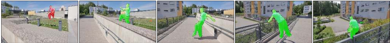
Figure 1. Example result of our technique: The segmentation of the first frame (red) is used to learn the model of the specific object to track, which is segmented in the rest of the frames independently (green). One every 20 frames shown of 90 in total.
