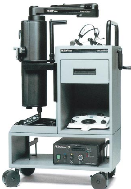
Figure 1. AESOP 2000 – an acronym for automated endoscopic system for optimal positioning as a voice-controlled robotic assistant for endoscopic surgery in its mobile carriage.
