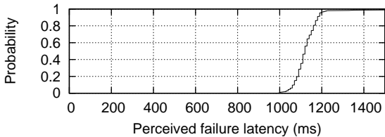
Figure 8: A CDF of the perceived communication disruption time between two hosts when an intermediate switch fails. These measurements include the one-second (application-configurable) keepalive timeout used by Onix. The hosts measure the disruption time by sending a ping every 10 ms and counting the number of missed replies.
