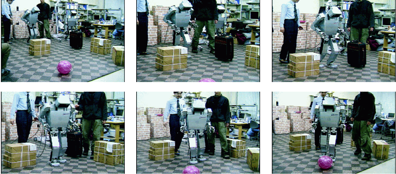
Figure 8: Snapshots of the humanoid H7 calculating and executing online the footstep sequence from Figure 1
