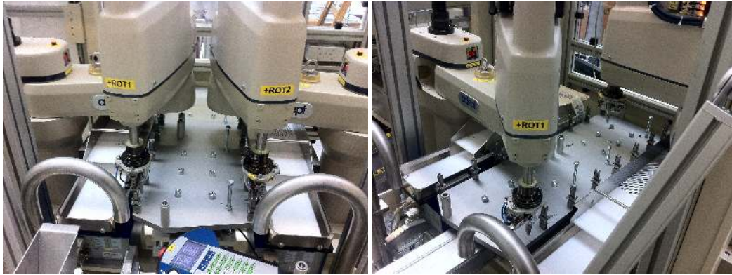
Figure 1.3: An industrial application: two robotic manipulators share the same work space.
