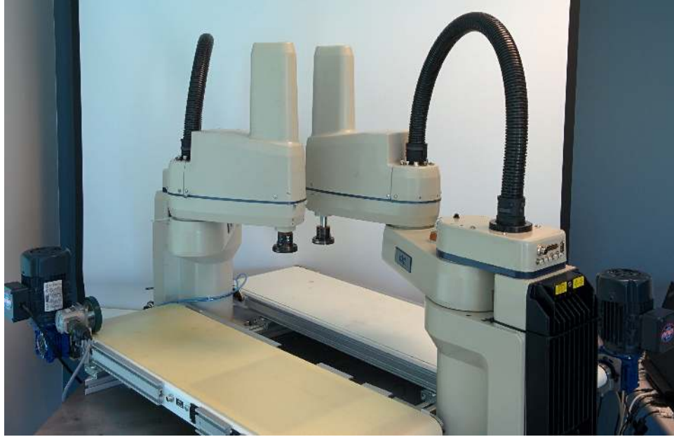
Figure 5.1: Experimental setup. Two Adept Cobra SCARA [1] robots sharing the same working environment.
