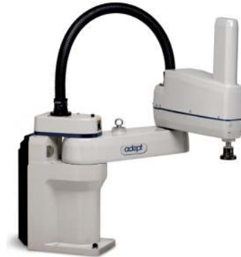
Figure 1.4: Cobra s600 SCARA Adept robot. Reprinted from [1]
