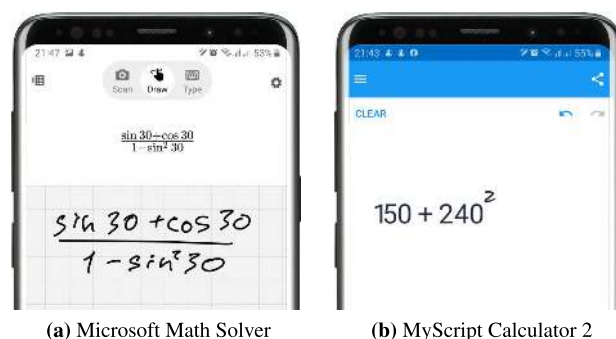
FIGURE 15. Examples of user interface: a) batch recognition and handwriting representation; b) iterative recognition and printed representation.
