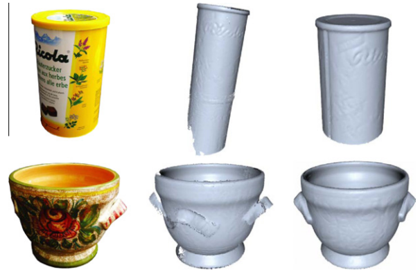
Fig. 11. Modeling results for textured objects. The middle column shows the artifacts that arise due to symmetries when only geometry is used for registration. The right column shows the correctly reconstructed objects when texture features are used for registration.
