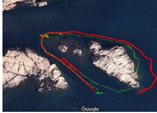
Figure 28: Vehicle’s trajectory (green) calculated by its dead-reckoning system and the camera’s trajectory (red) estimated by the image-based reconstruction. Both trajectories are shown overlapped with a satellite image of the test scenario (Map data ©2017 Google).
