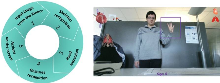
Fig. 2. Architecture of the gesture recognition system (left) and user interface (right)
