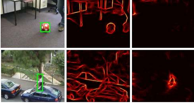
Figure 3. Two examples of edge and motion boundary responses. In each row, from left to right, we show the original image (with the object in a green box), edges and motion boundaries. The edges provide a stronger response in the example in the first row while motion boundaries are more effective in the example in the second row.
