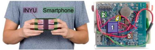
Fig. 1. INYU sensor and prototype. Front: 1: STM32L151RDT6 (ARM Cortex-M3 MCU, 384 KB Flash, 48 KB RAM), 2: MPU-6000 (6-axis I^2C motion sensor), 3: nRF8001 (Bluetooth low energy v4.0 radio). Back: 4: ADS1191 (Analog front-end for ECG applications).
