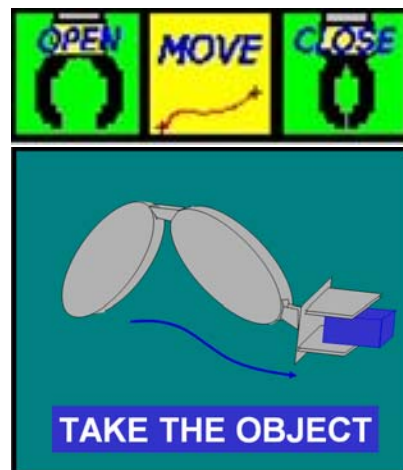
Figure 16: An example of an icon that can belong to the Macro Repository area: the TAKE-THE-OBJECT icon. Using Movement and Flow icons, user must insert a minimum of three icon in the Program Score ( up ): OPEN, MOVE TO and CLOSE. Using a Macro icon of this program ( bottom ), user will add only an icon to the Program Score, and will specify the (relative or absolute) position of the object.
