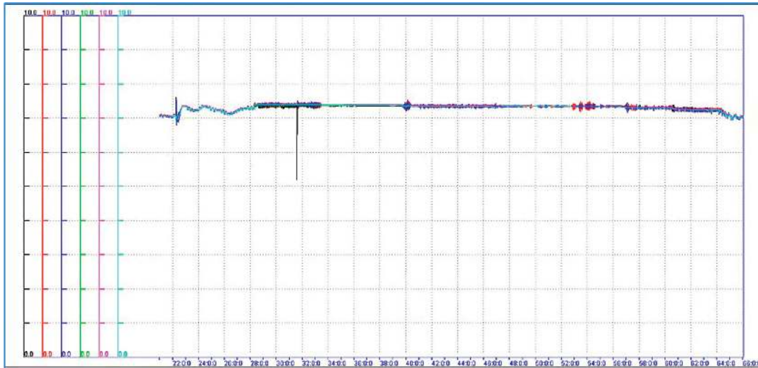
FIGURE 16: Steam generator level transient—pressures. Steam generator pressures (black, red, blue & green, magenta, cyan), range: 0~10 MPa.
