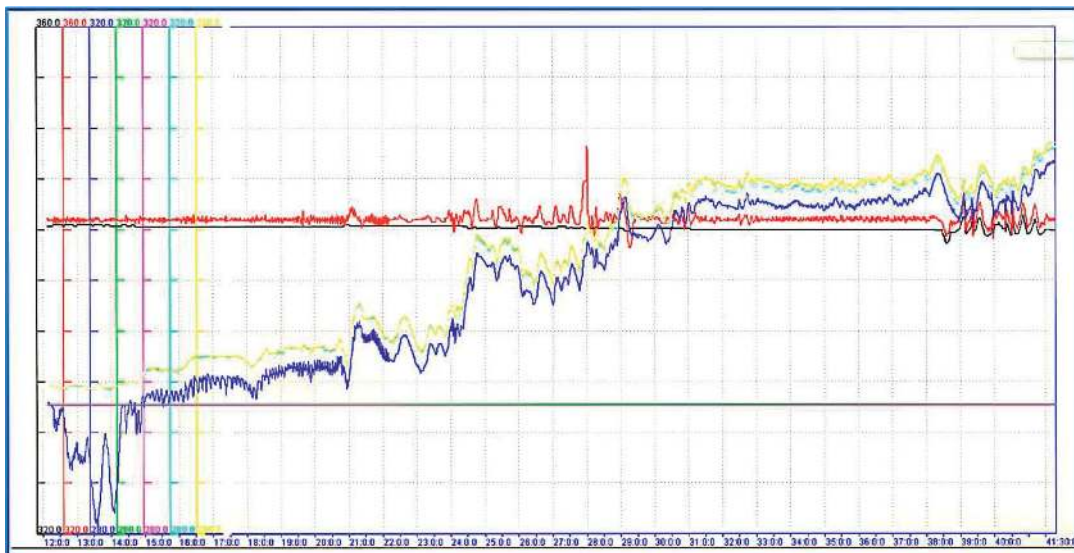
FIGURE 6: Power up operation—temperatures. Pressurizer steam space temperature (black & red), range: 320~360°C; Reactor circulation loop average temperatures (blue, green, magenta & cyan, orange, white), range: 280~320°C.
