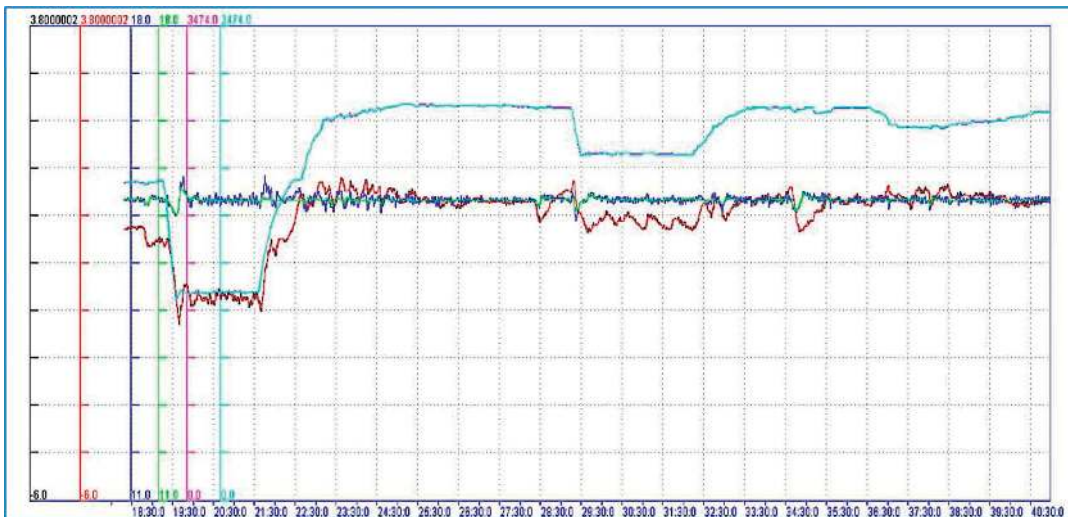
FIGURE 9: Power maneuvering—power, pressure, and level. Reactor thermal power (magenta & cyan), range: 0~3474 MW; pressurizer pressure (blue & green), range: 11~18 MPa; pressurizer level (black & red), range: -6~3.8 m.
