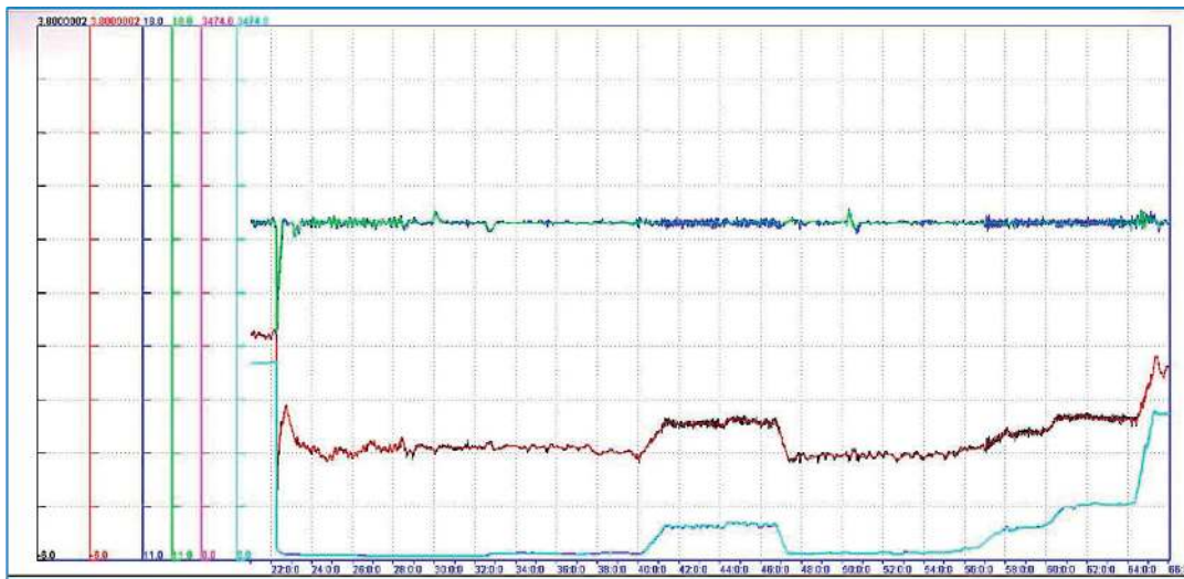
FIGURE 14: Steam generator level transient—power, pressure, and level. Reactor thermal power (magenta & cyan), range: 0\sim 3474 MW; pressurizer pressure (blue & green), range: 11\sim 18 MPa; pressurizer level (black & red), range: -6\sim 3.8 m.
