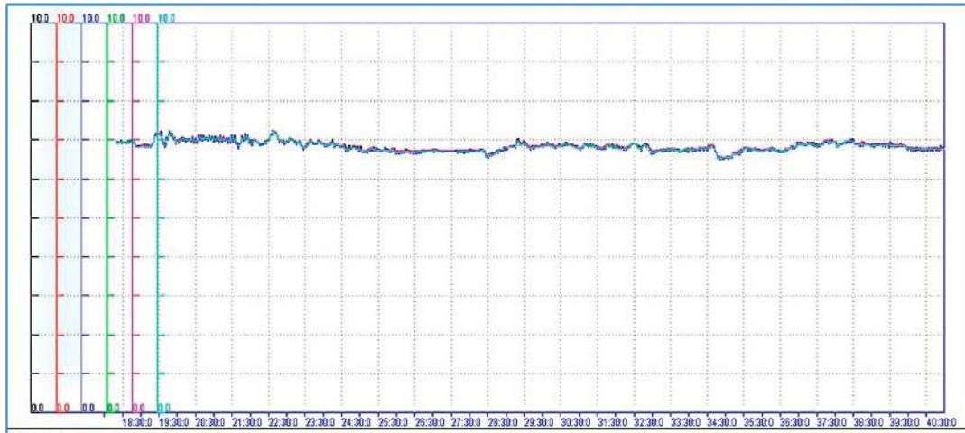
FIGURE 11: Power maneuvering—pressures. Steam generator pressures (black, red, blue & green, magenta, cyan), range: 0~10 MPa.
