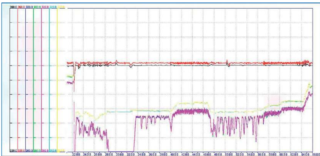
FIGURE 15: Steam generator level transient—temperatures. Pressurizer steam space temperature (black & red), range: 320\sim 360^{\circ}\text{C} ; reactor circulation loop average temperatures (blue, green, magenta & cyan, orange, white), range: 280\sim 320^{\circ}\text{C} .
