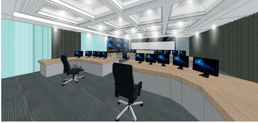
FIGURE 1: Control room mimic of digital I&amp;C validation real-time simulation platform.
