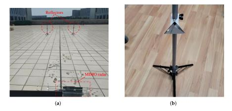
Figure 7. Measurement scenarios. (a) Locations of MIMO radar and corner reflectors, (b) corner reflector.
