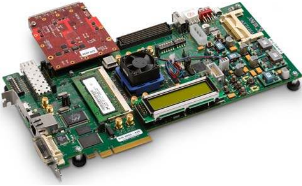
Fig. 4. Xilinx ML605 board with Virtex 6 FPGA chip and 4DSP FMC150 daughter card (FMC150 and FMC151 cards look practically the same).
