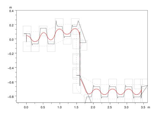
Figure 3: Foot step placement and ankle motion (grey), Center of Pressure (black) and Center of Mass (red) positions for the sample motion described in Section 6, obtained with the Predictive Control scheme (19), but with  $\gamma = 0$ .
