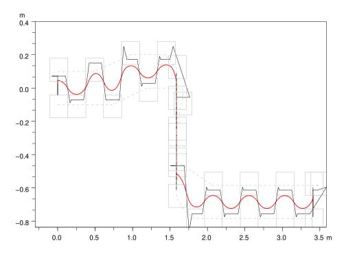
Figure 5: Foot step placement and ankle motion (grey), Center of Pressure (black) and Center of Mass (red) positions for the sample motion described in Section 6, obtained with the Predictive Control scheme (19).
