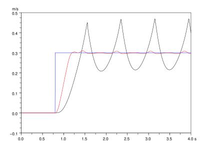
Figure 7: Comparison between the forward speed obtained with our method (red) and with the method proposed in [11] (black) when the reference speed (blue) is changed from 0 to 0.3 ms<sup>-1</sup> at the beginning of a step.
