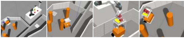
Figure 2: Scenario 1 - A mobile robot navigates towards a docking station next to a manipulator robot, which picks up some pieces from a table and places them on the mobile robot. The mobile robot comes back.
