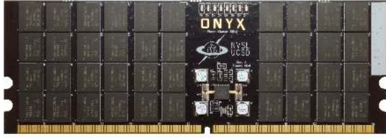
Figure 2: The Onyx PCM DIMM The PCM DIMM contains eight identical ranks of five chips. Ranks share data lines, and all chips share address lines.
