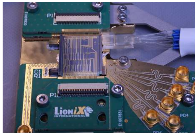
Fig. 8. Commercial example of TriPleX waveguide technology: Integrated Optical Beam Forming network showing hybrid integration of TriPleX and InP elements into an MWP module for satellite communications.
