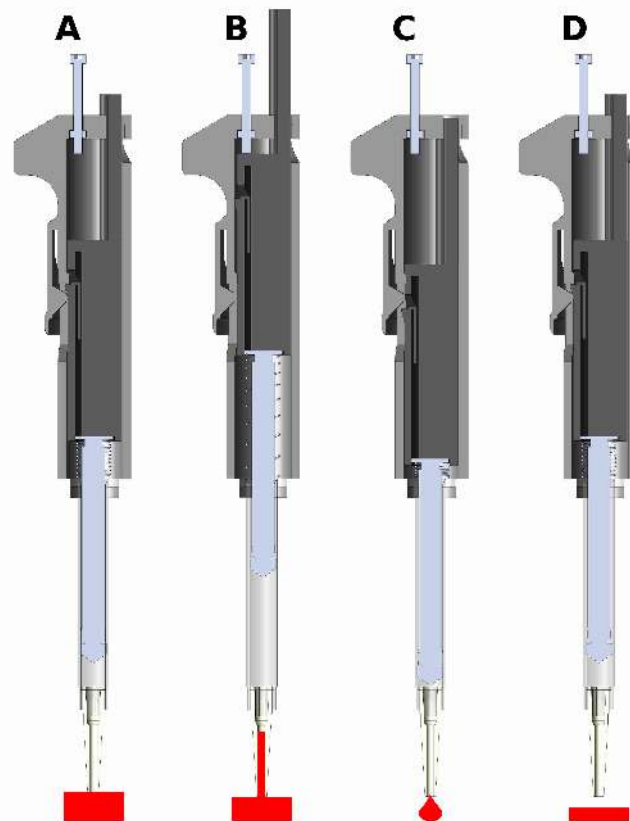
Figure 2. CAD renderings of assembled pipette and function. The pipette actuates the syringe to three positions. (A) The latched position. When the plunger is pressed, the pipette locks at this position. The tip is then placed in a liquid, and the unlatching button is pressed to release the pipette back to the set position (B), drawing in liquid. (B) The set position. The position of the screw determines the total displacement that the plunger moves. The pipette is spring loaded to return to this position. (C) The blow-out position. The fluid is transferred by pressing the plunger past the latched position to blow-out all the liquid. (D) Return to the latched position. The pipette returns to the latched position ready to perform another transfer.
