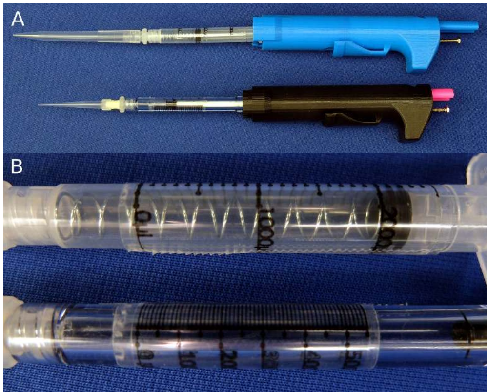
Figure 4. Photos of assembled pipettes. (A) Two assemblies of the pipette: the 100–1000- \mu\text{L} configuration (top) and the 30–300- \mu\text{L} configuration (bottom). (B) Close-up photo of the taped on scale for each of the syringes. Scales are available in the Appendix A: Figures A1 and A2.
