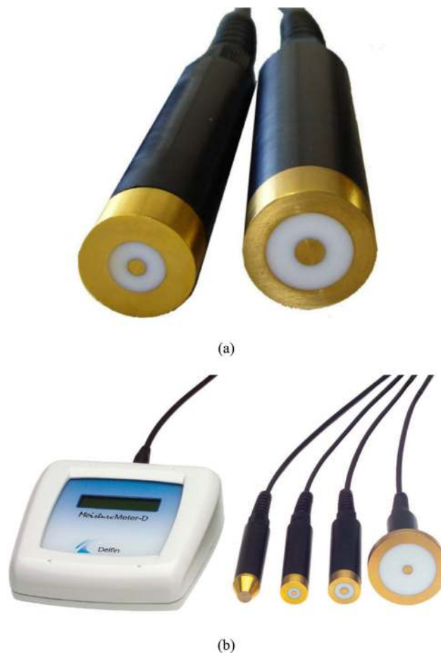
Fig. 1. Photographs of (a) the two probes used in this experiment, and (b) the complete measurement system.
