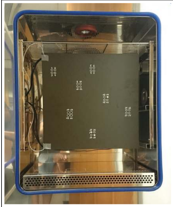
Figure 11. Photograph of the “SHM plate” in the climate chamber, where the tests were performed at 23°C and 50% RH. Two temperature sensors were installed on the top left and bottom left to measure the surface temperature of the samples.
