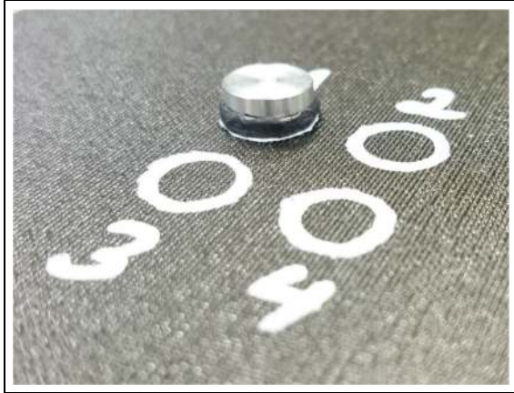
Figure 7. Photograph of the reversible damage model in the form of an aluminum disk with a diameter of 10 mm coupled to the structure by tacky tape. White circles indicate four closely spaced damage positions (cf. Figure 12).
