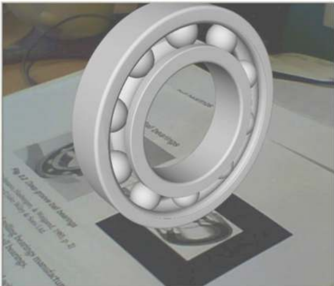
Fig. 1 Computer screenshot of a virtual ball bearing superimposed over a real 2-D image
