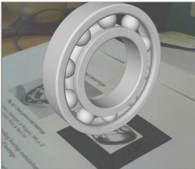
Fig. 2 An image of a roller bearing, viewed on a computer screen via a webcam focused on the augmented reality target
