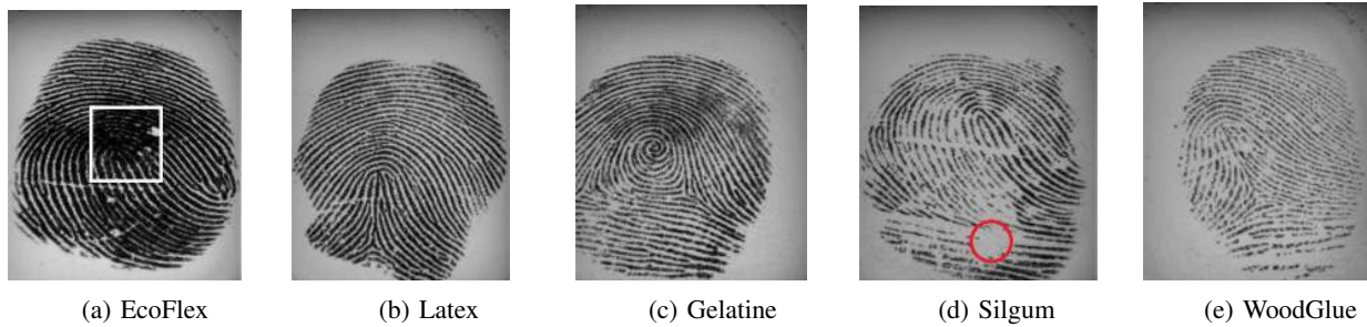
Fig. 2: Examples of fake fingerprint images (from the LivDet 2011 [48] database) corresponding to five different fabrication materials. The artifacts introduced (examples indicated by the circle and square) are typically quite prominent for silgum, wood glue and ecoflex materials.
